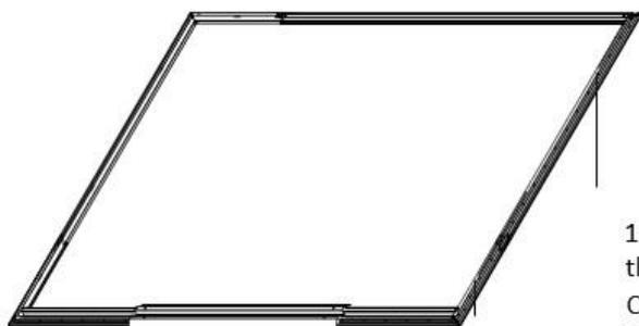
1. When diagonal measurements are equal, the frame is square.
